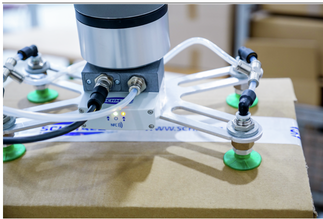
Pneumatic vacuum generator RECBi when handling cardboard boxes
